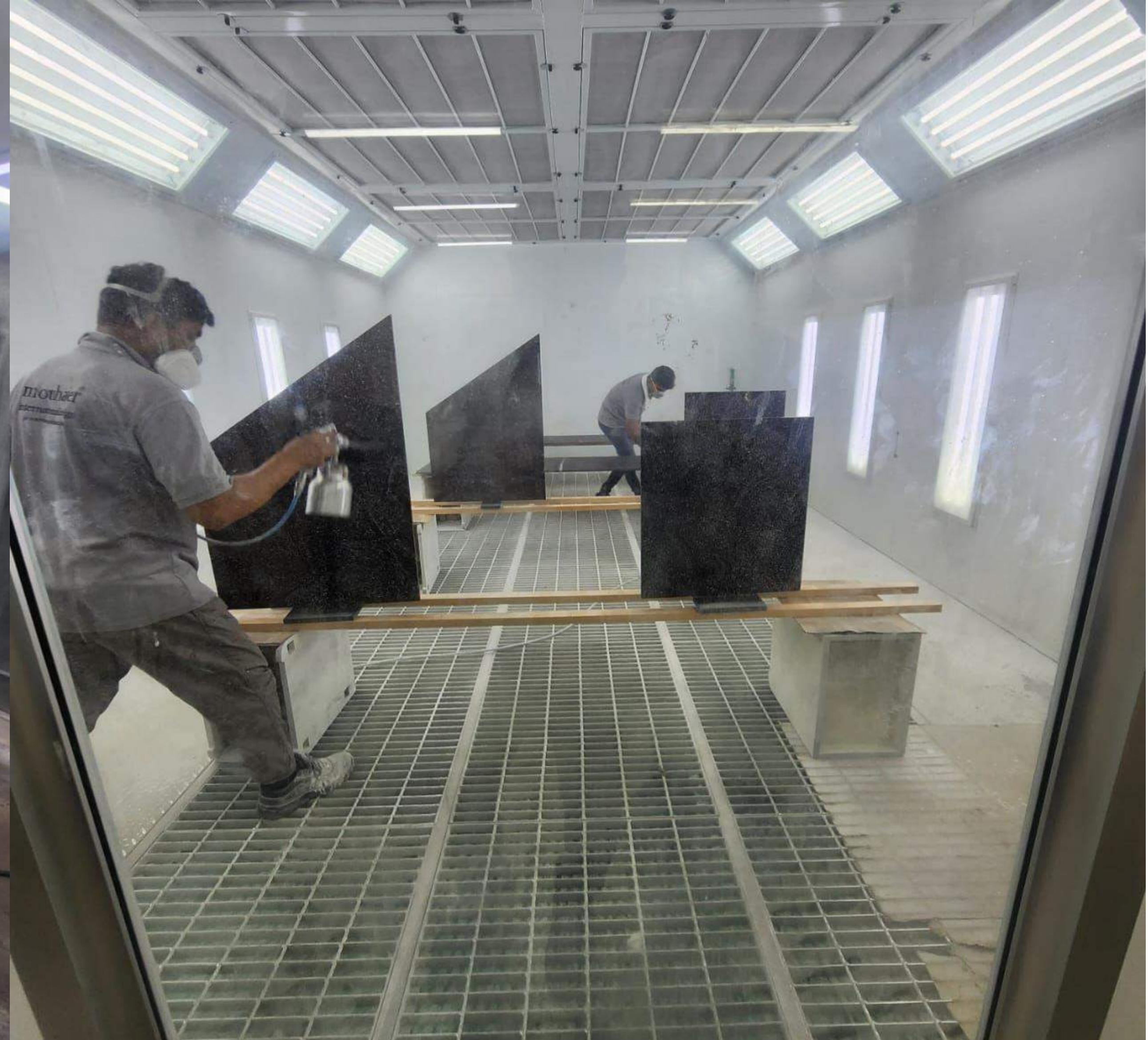
The Paint Booth where high-powered ventilation system for lighting & temperature control is provided for strict quality measures during painting items.
